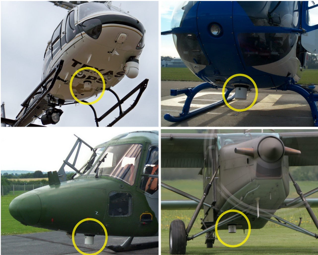
Fig 45) Antenna Installed in Good Locations
