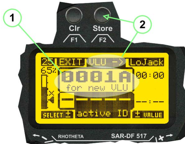
Fig 34) LoJack Scan Mode with new VLU Code received
