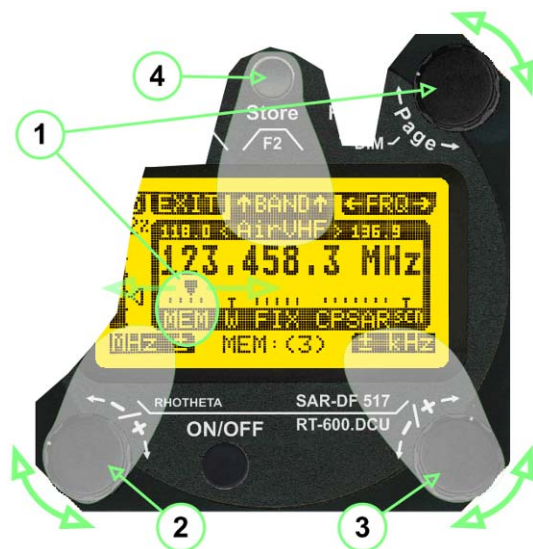
Fig 15) Recall frequency of Memory channel 3
