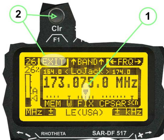
Fig 32) FRQ Selection Page, FRQ = LoJack, BAND = LoJack (164-174 MHz)
