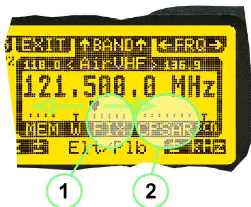
Fig 16) FRQ Selection Page with FIX1 selected
