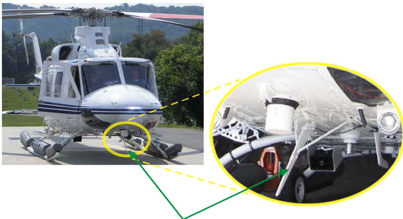
Fig 44) Antenna Installed in a Bad Location
