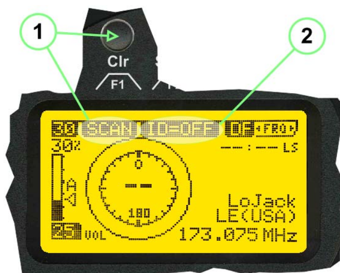
Fig 33) DF Mode with LoJack filter OFF
