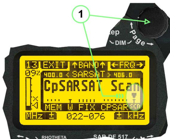
Fig 25) FRQ Selection Page with SCN COSPAS-SARSAT Scan Page selected
